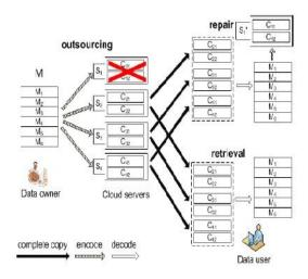
Fig 2: storage systems based on optimal erasure codes
