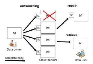
Fig 1: storage systems based on replication.
